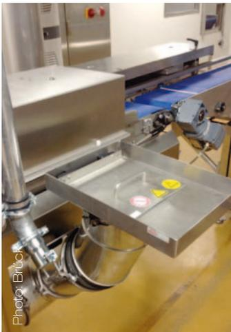
Right photo: The manual feed station for bread residues is also equipped with a vacuum cleaning connection and connected to the overall system via a pipe connection.
