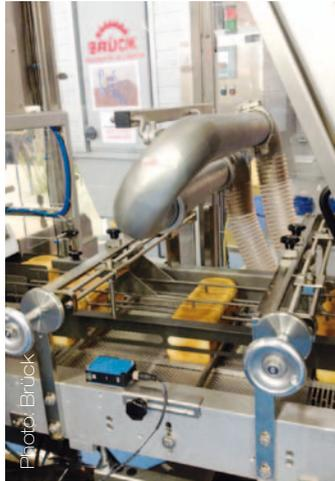
Left photo: Any crumbs which occur during cutting in the slicer and which are transported upwards by the slicers are caught by the vibrating tray. Middle photo: After cutting in the slicer the over-suction unit removes any remaining bread crumbs on the surface.
